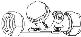
**E960086NU**. Brass valve with isolating & filter only features. 15mm compression fittings at both ends. Supplied in pairs.
