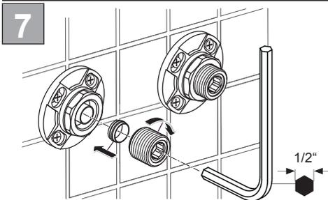
Fit the olives to the pipes prior to screwing the two 3/4" connectors into the wall mount plate using a 1/2" allen key. The connectors will have to be securely screwed in to form the necessary compression joint between the olive, wall plate and connector. Retain the brass adaptors with a spanner when making the compression joints.
