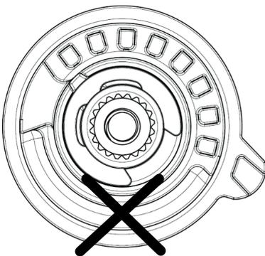
**No temperature-stop fitted gives full hot supply temperature, upwards of 65°C. NOT RECOMMENDED!**
