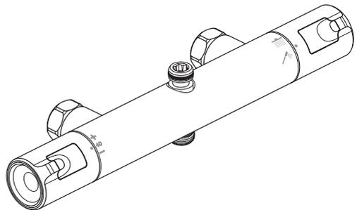
Shower valve shown without wall mounting brackets assembled. Mixer supplied with **A7225AA**. Right side handle controls flow & diverts between dual shower outlets. Product is supplied with the dual shower pack shown on the previous page.
