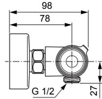
Basic bar shower mixer dimensions shown with wall mounting brackets assembled
