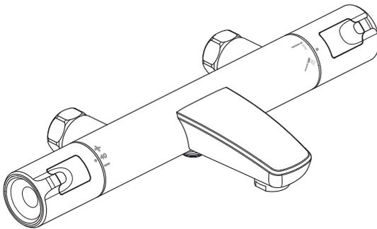
Wall bath/shower mixer shown without wall mounting brackets assembled. Mixer supplied with **A7697AA** product. Right side handle controls flow & diverts between bath fill & shower hand set. Note: **A7224AA** is supplied without a shower kit.
