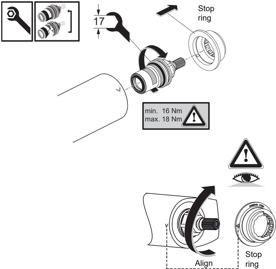
1. Observe disassembling sequence, as detailed in **section 14, steps 1 to 3.**
