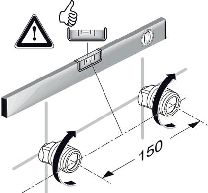
Pre-installation: Pipework should be run in or behind the solid wall, terminating with G1/2" female nipples securely fastened at 150 centres.
