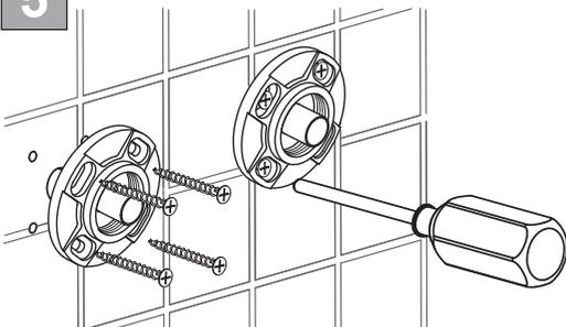
Apply a smear of silicone sealant to the rear of the assembled brackets and push them over the pipework.
