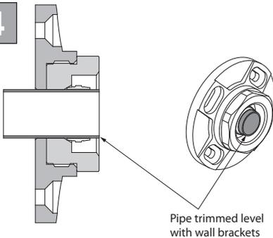
The pipes should be trimmed level to the wall bracket. If using a pipe cutter it will be necessary to mark the pipes and then remove the bracket before trimming to its correct length.
