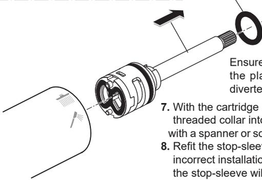
Ensure these locator pins are correctly located into the plastic moulding inside the mixer body. The diverter will then drop down to the correct depth.
