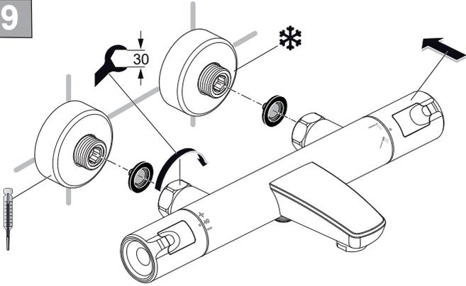
As with the bar shower mixer, the wall mounted bath/shower mixer is assembled to the wall brackets in the same way to complete the installation.
