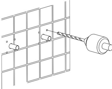
Drill holes appropriate for your choice of fixings into the wall.
