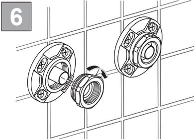
Screw the brass adaptors over the pipes into the plastic brackets. 36mm A/F Spanner flats are provided, hand tightness is adequate.
