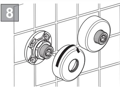
When the sealant has set, fit the covers by screwing them onto the adaptors until they are flush with the wall.
