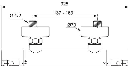
Dimensions are in millimetres & may vary within permitted tolerances
