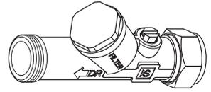
Spares code **E960613NU** contains a pair of combined service valves. Include a flow regulator, check valve, strainer mesh (filter) & isolating valve. The flow regulator and check valve can be removed if not required.
