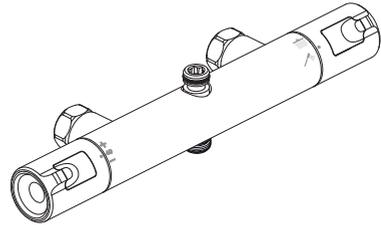
**A7227AA** Shower valve shown without wall mounting brackets assembled. Right handle controls flow & diverts between hand spray & overhead rain shower. Includes dual shower pack shown below.
