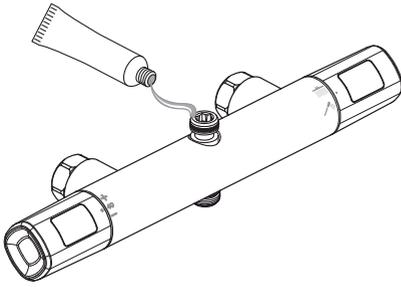
Note: the mixers supplied with A7225AA & A7227AA are fitted with an additional outlet nipple on the top surface to connect the over head shower plate.
